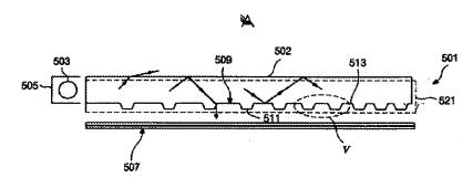
Figure 4 depicts an auxiliary light source device, including a light source 503, a lamp reflector 505, a light directing member 501 having an upper surface 502, a lower surface 509, a wall reflector 521, a plurality of convex portions 511, a surface 513, and a reflector 507. (Spec. 6, Il. 5-27).
